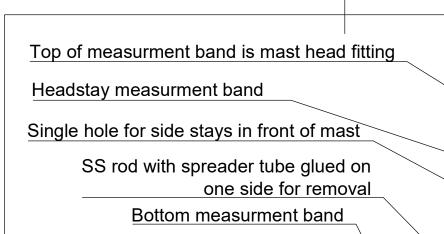
Mast rake measurment G is deck hight to bottom jib band
